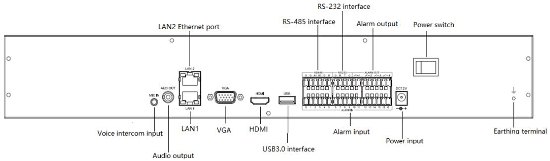
The interfaces on the rear panel of 1099/455 are shown as below:
