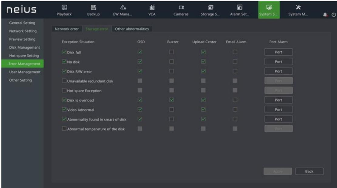
2.If exceptions are checked, the corresponding linkage actions of the system, including screen display, voice prompt and upload center, can be checked when these exceptions occur.
