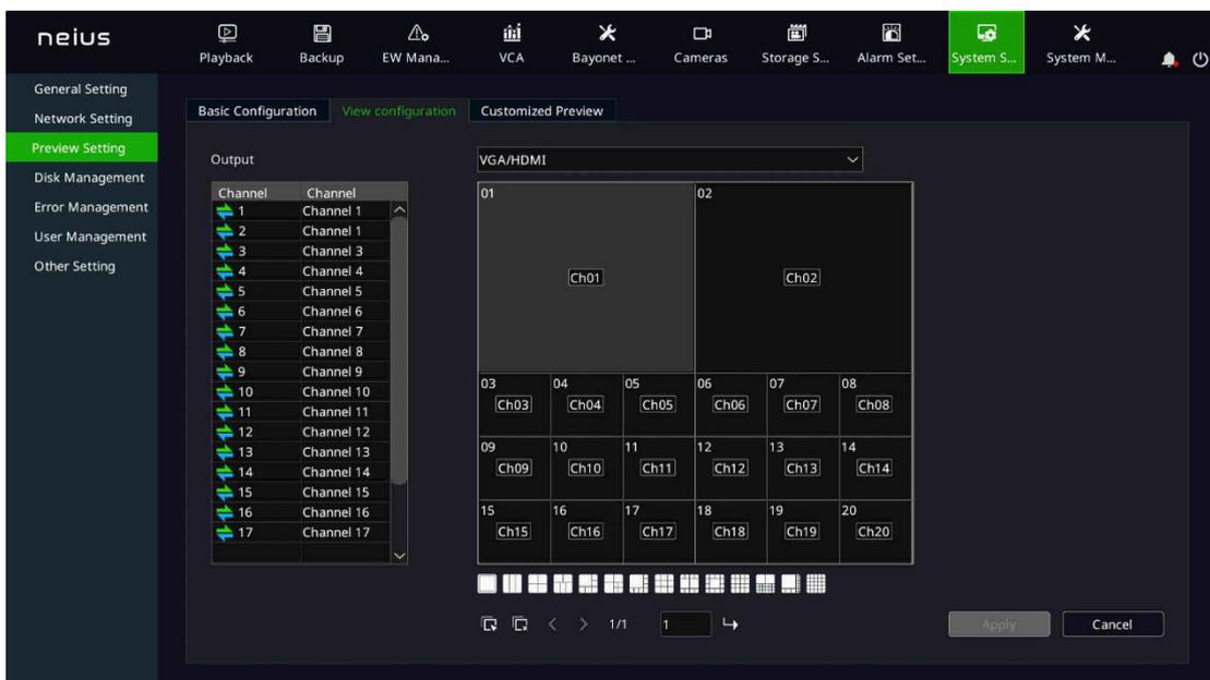
Select the screen number on the right, double-click the screen to delete the preview channel, and double-click the channel number in the table on the left to configure the channel number to the specified location. To open or close all preview channels, click Auto Configure and Clear All on the lower right.
