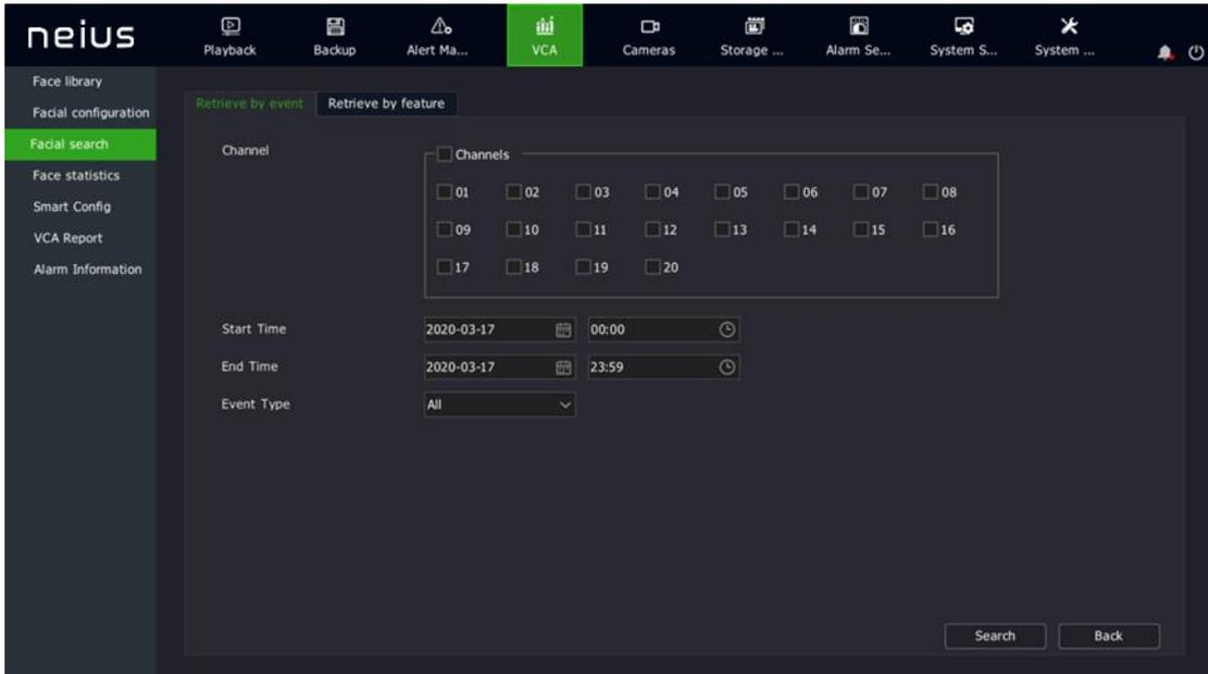
"Retrieve by Event": Users can choose the corresponding channel, and set the statistical type for the channel(options include all, face detection, comparison alarm, stranger alarm, frequency alarm, and stay alarm) to retrieve the corresponding type of data.
