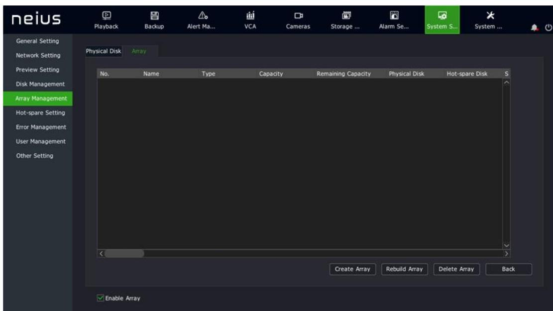
2. Create an array. Click the "Create Array" button to enter the Create Array interface, as shown in the figure below. To create an array, you must specify a array name, array type, physical disk that makes up the array, and the hot standby disk number. When all the information is set, click the OK button to start creating the array.
