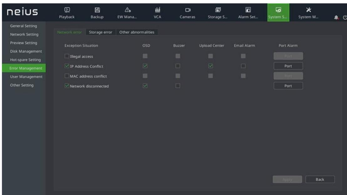
2. If exceptions are checked, the corresponding linkage actions of the system, including screen display, voice prompt and upload center, can be checked when these exceptions occur.
