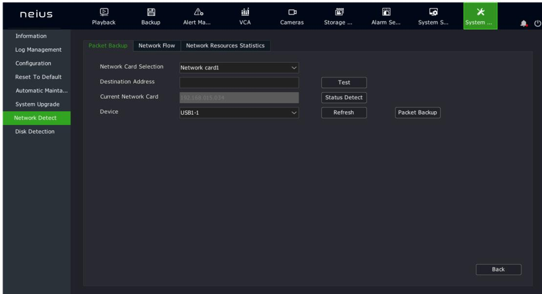
2. In the network testing field, enter the destination address to test whether the address can be pinged through.
