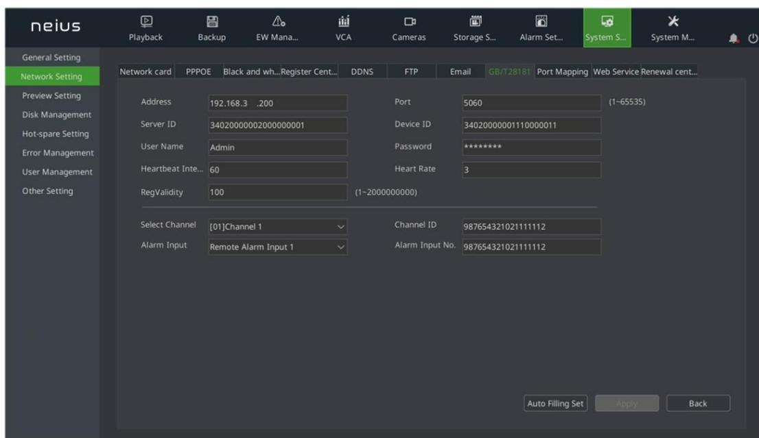
2. Input address, server ID, account, heartbeat interval, registration validity, port, device ID, password, heartbeat times, channel selection, channel number, alarm input, alarm input number.
