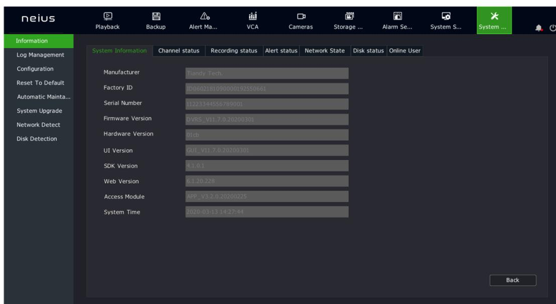
2. The manufacturer, serial number, kernel version, hardware version, SDK version, webpage version, UI version, and system time can be checked under System Info.
