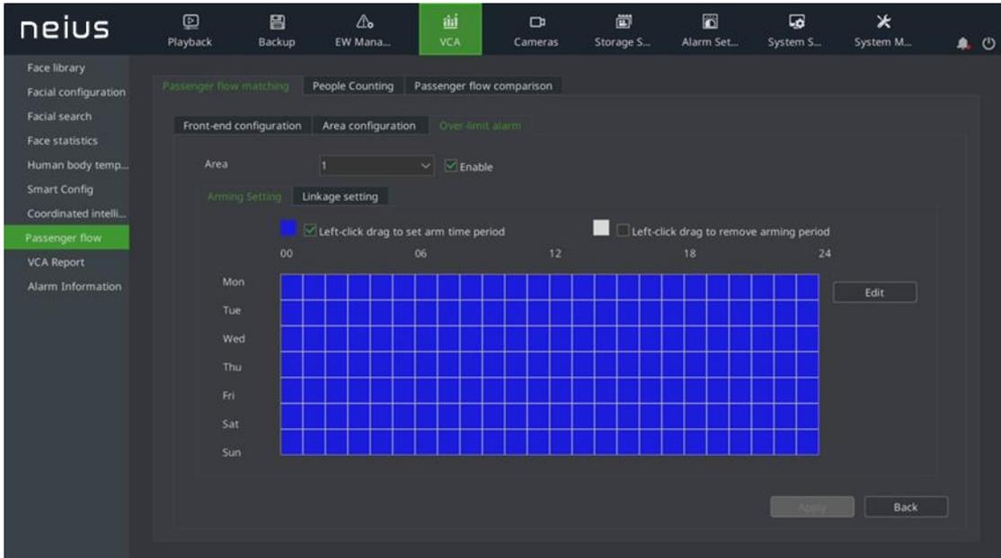
2. Select the linkage area to set the alarm time period and linkage method. The linkage methods support the front-end sound alarm and output port, as shown in the figure below:
