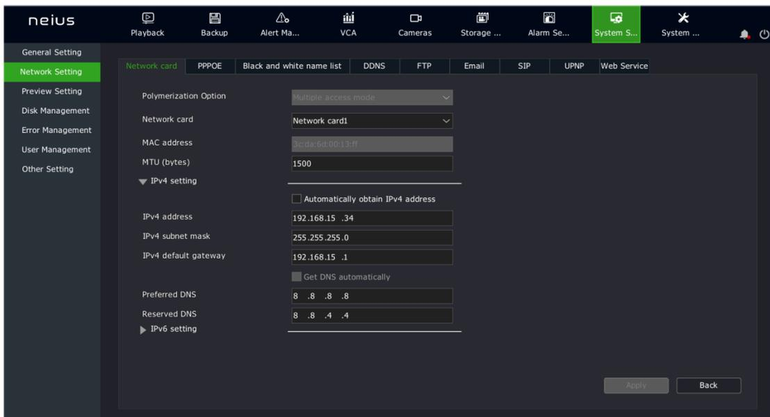
2. Choose to automatically obtain or manually set the IP address. If auto obtain is selected, the system will automatically obtain the IP address from the DHCP in the network.
