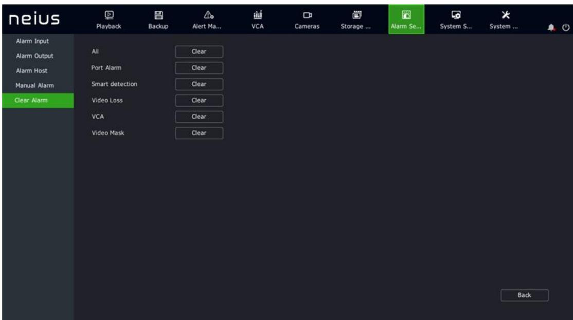
2. Select the alarm type to clear from the manual clearing interface. Options include "All", "Port Alarm", "Motion Detection", "Video Loss", "Intelligent Analysis", and "Video Occlusion". Click the corresponding button to clear this alarm type.
