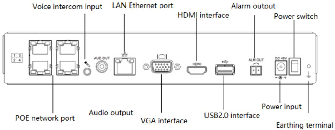
The interfaces on the rear panel of 1099/407P (the NVR has also the Alarm IO that is not reported) are shown as below:
