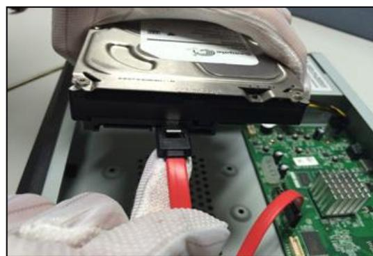
3. Connect one end of the HDD power cable to the SATA interface of the NVR master board, and the other end to the HDD.
