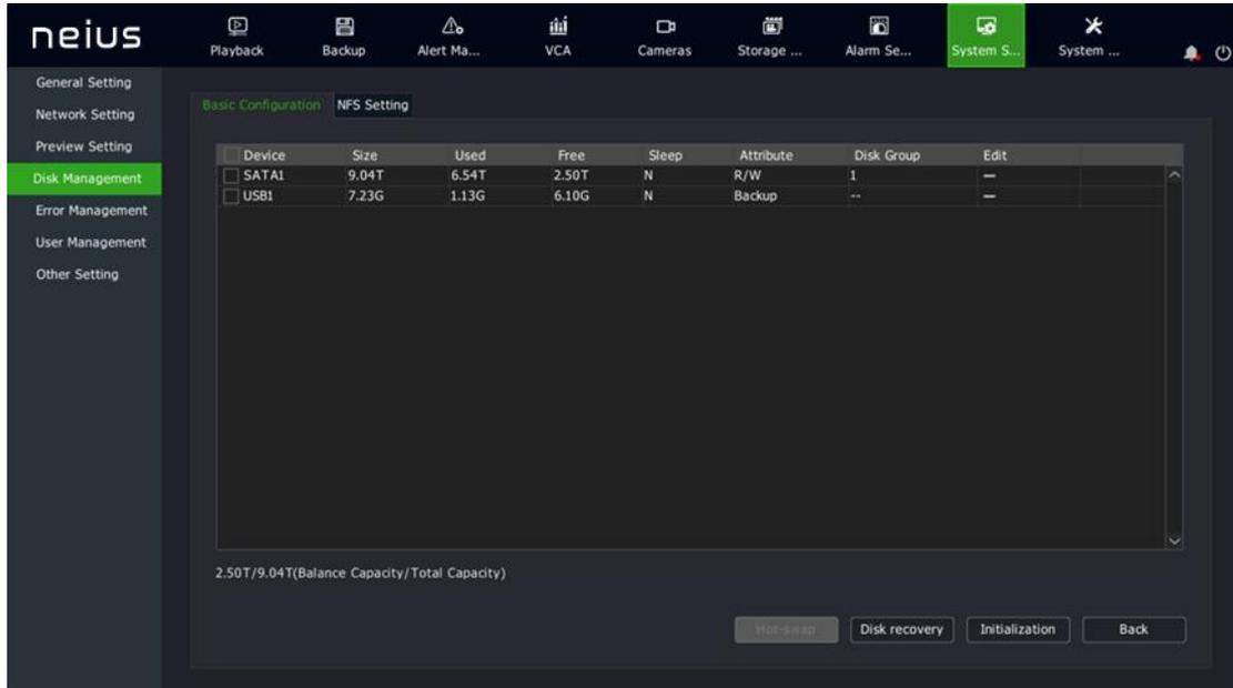
2. The interface can display the total remaining capacity and total capacity of the current HDD and virtual disk.
