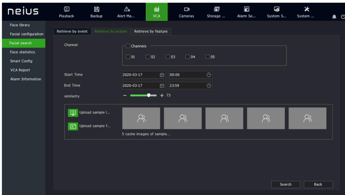
"Retrieve by Picture": Users can select the corresponding channel, and set the channel number, similarity and sample picture, and then click the "Retrieve" button to filter out alarm pictures of the corresponding similarity from all the alarm pictures.
