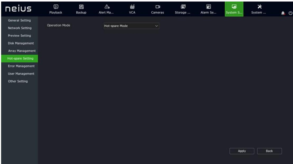
3. Click the "Apply" button, and the system prompts that the device needs to be restarted to make the setting effective.
