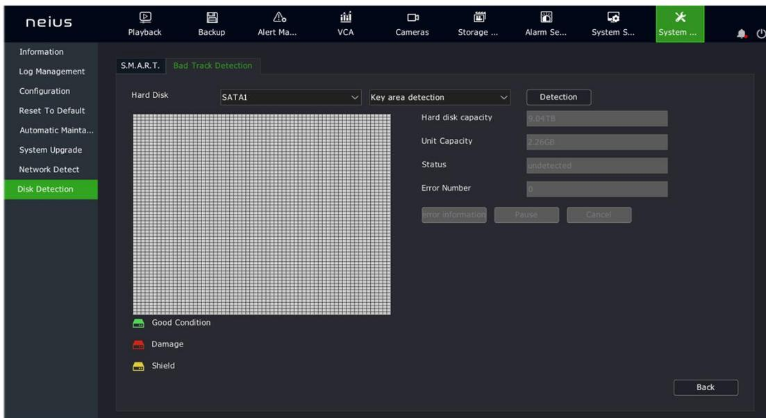
2. Select the hard disk and detection method and click the Detection button to enter the detection status.
