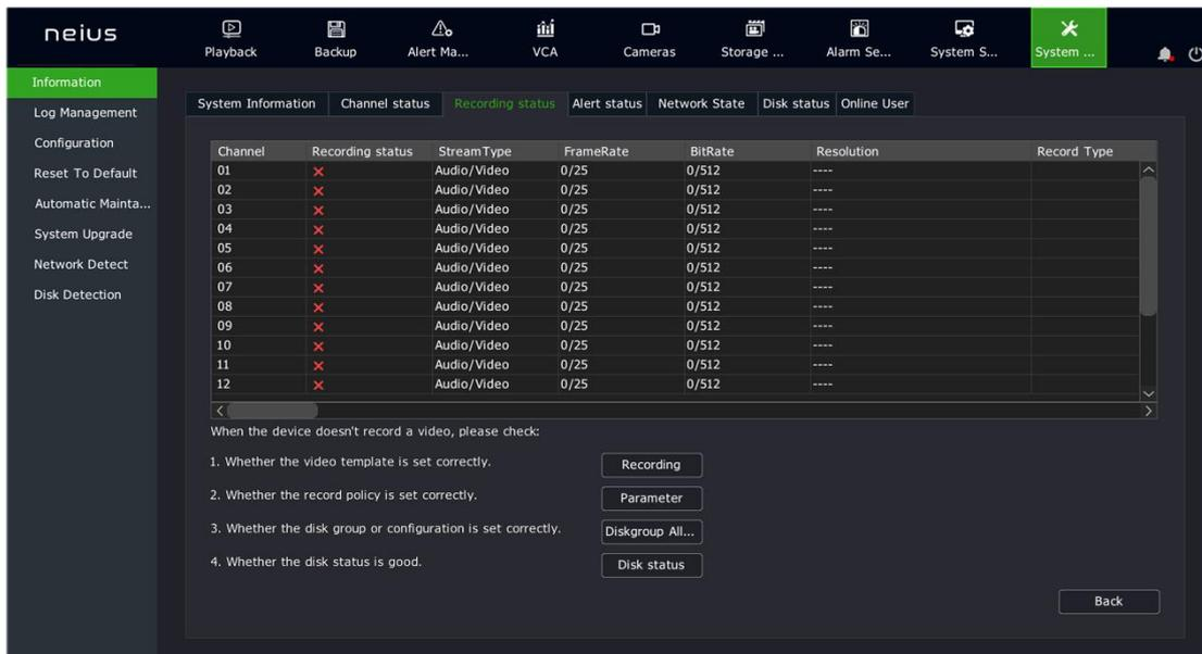
2.Channel number, recording status, stream type, real-time frame rate/set frame rate, real-time bitrate/set bitrate, video resolution, video type, compression parameters, redundancy status can be checked under Record Status.
