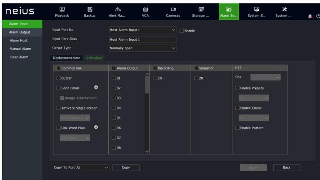
2. Select the input port number to set. On the interface, users can set local and host alarm input port numbers.
