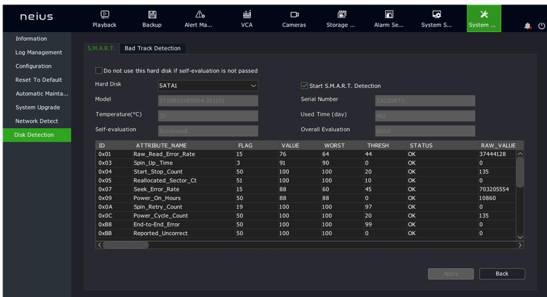
2. Select the disk to detect and check "Enable S.M.A.R.T Detection" to enable the S.M.A.R.T detection function of the disk. S.M.A.R.T detection information is displayed in the corresponding interface.
