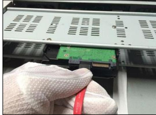
3. Connect the power cable to the hard disk, attach the top cover of the chassis and fix it with screws.
