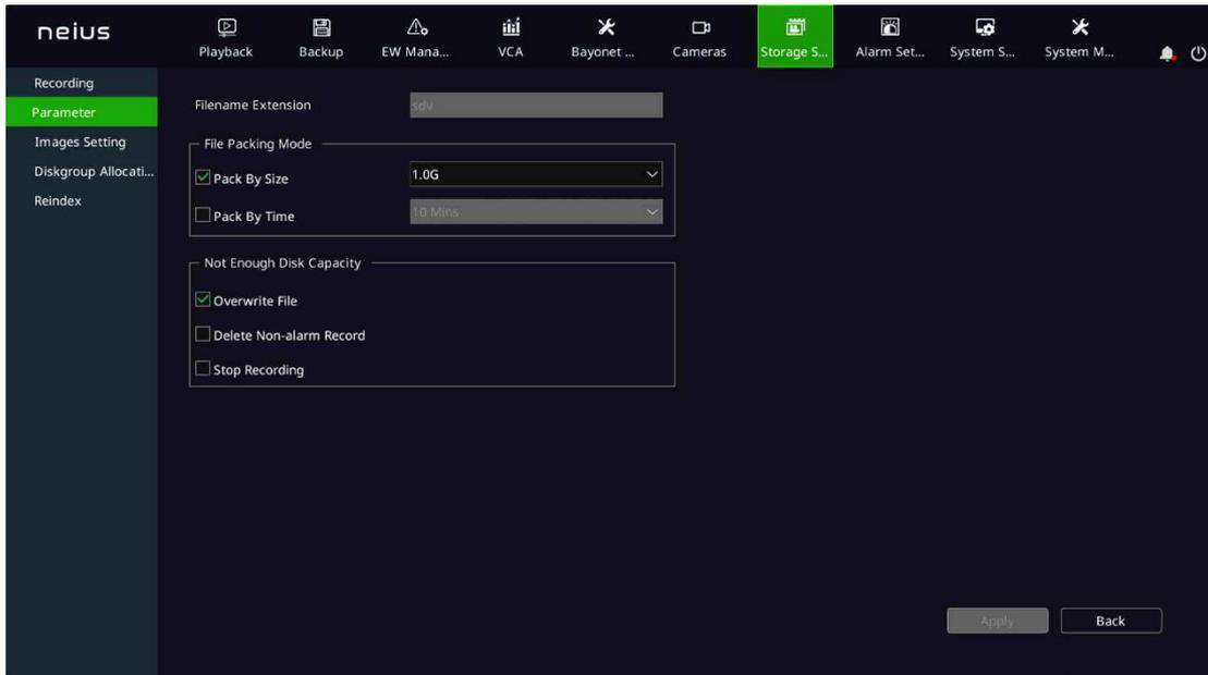
2. Select the processing method of the system when the disk space is insufficient, such as "Overwrite Files", "Delete Non-alarm Record" or "Stop Recording".
