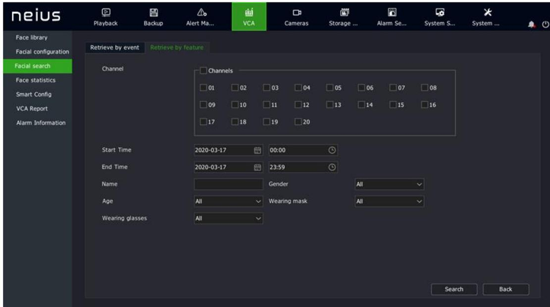
"Retrieve by Feature": Users can select the corresponding channel, set the channel name, gender, age, glasses and mask, and click the "Retrieve" button to filter out the alarm pictures of the corresponding features from all the alarm pictures.
