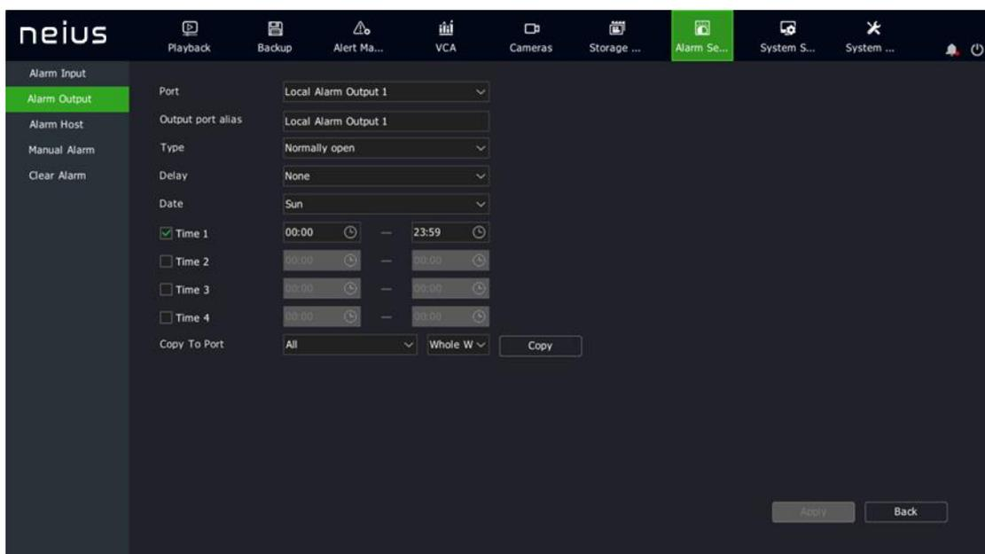
2. Select the output port number to set. On the interface, users can set the local and host alarm output port numbers.
