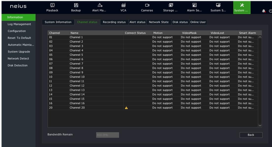
2. Channel number, channel name, connection status, motion detection status, video occlusion status and video loss status can be checked under Channel Status.
