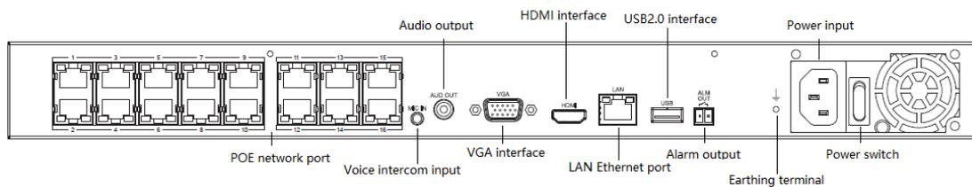
The interfaces on the rear panel of 1099/454 are shown as below:
