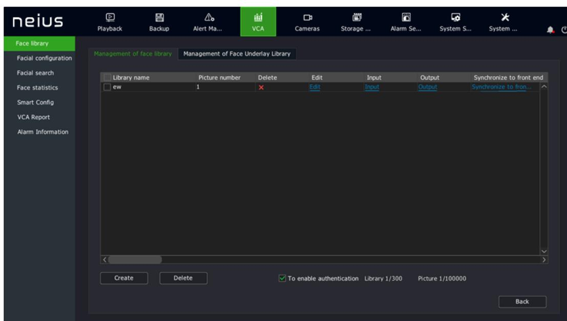
2. The existing face database data can be retrieved from the face database management and the face image library can be managed by using buttons such as "Create" and "Delete". As well, the face library data can be operated with [Import] and [Export], and [Synchronize to Front End] and other operations.
