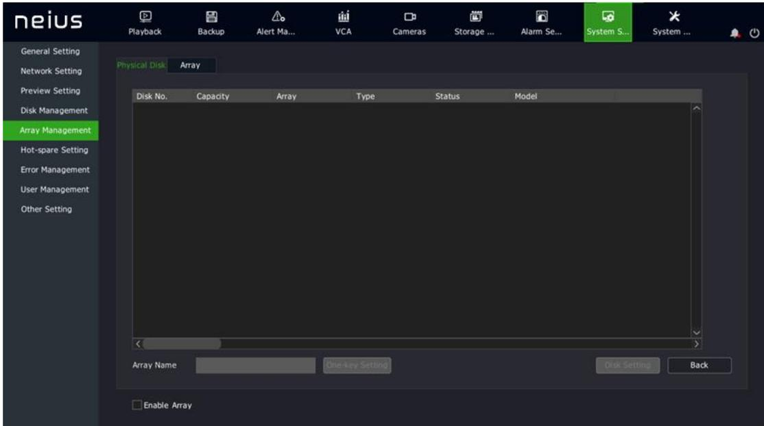
2. Enable array. Check "Enable Array" and the operation will take effect after reboot.
