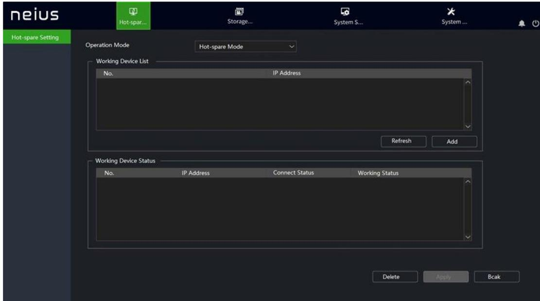
6. Click the "Refresh" button to display active units with hot standby function enabled in the active unit list. Select the active unit to set hot standby mode.
