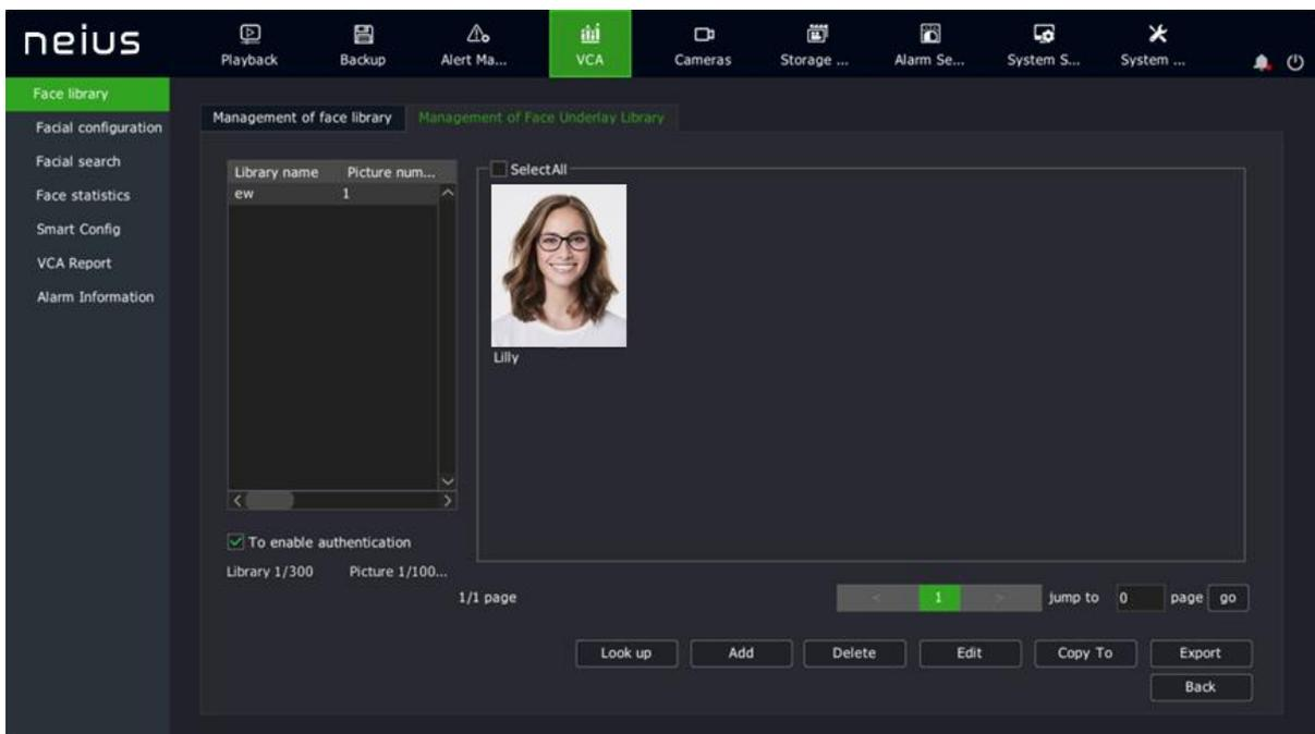
2. Base image management of the face database. The original face images are the basis of face recognition algorithm. Users can use the following buttons to manage the base images.
