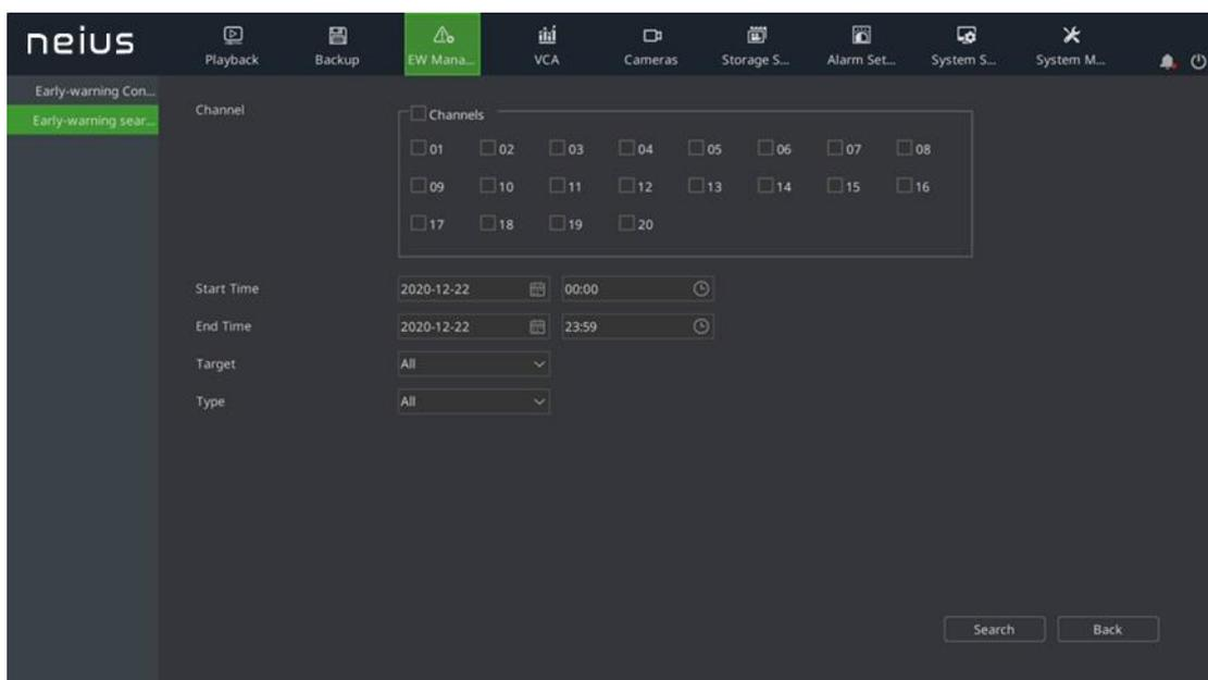
2. Retrieval targets are divided into all, people, cars and others; types are: all, tripwire, perimeter - intrusion, perimeter - departure. Select the corresponding target and type and
