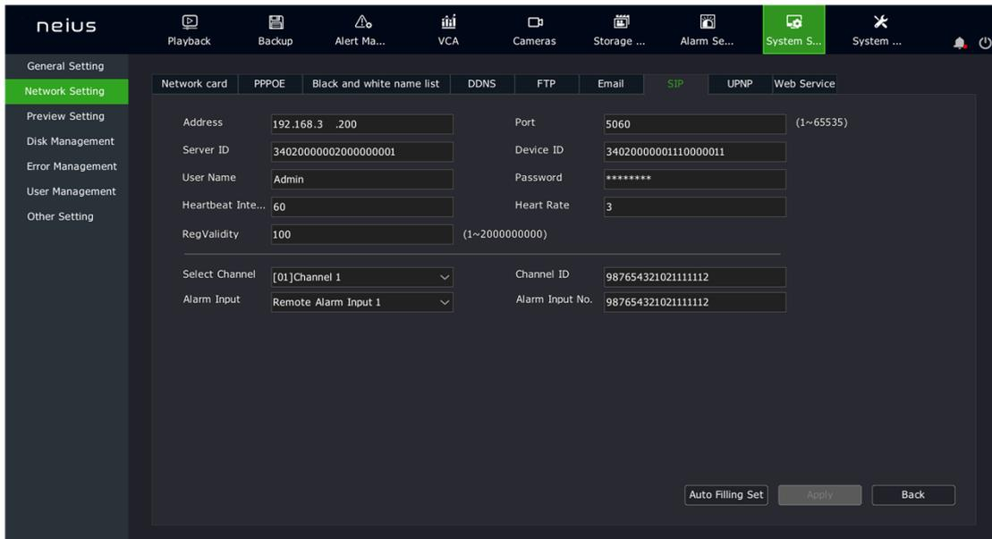
2. Enter address, server ID, account, heartbeat interval, term of validity, port, device ID, password, heartbeat rate, channel selection, channel number, alarm input and alarm input number.
