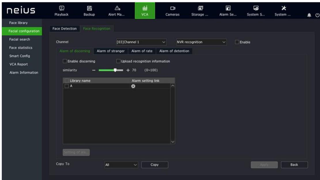
2. Select the algorithm type for face recognition, and choose to enable IPC Recognition/NVR recognition.
