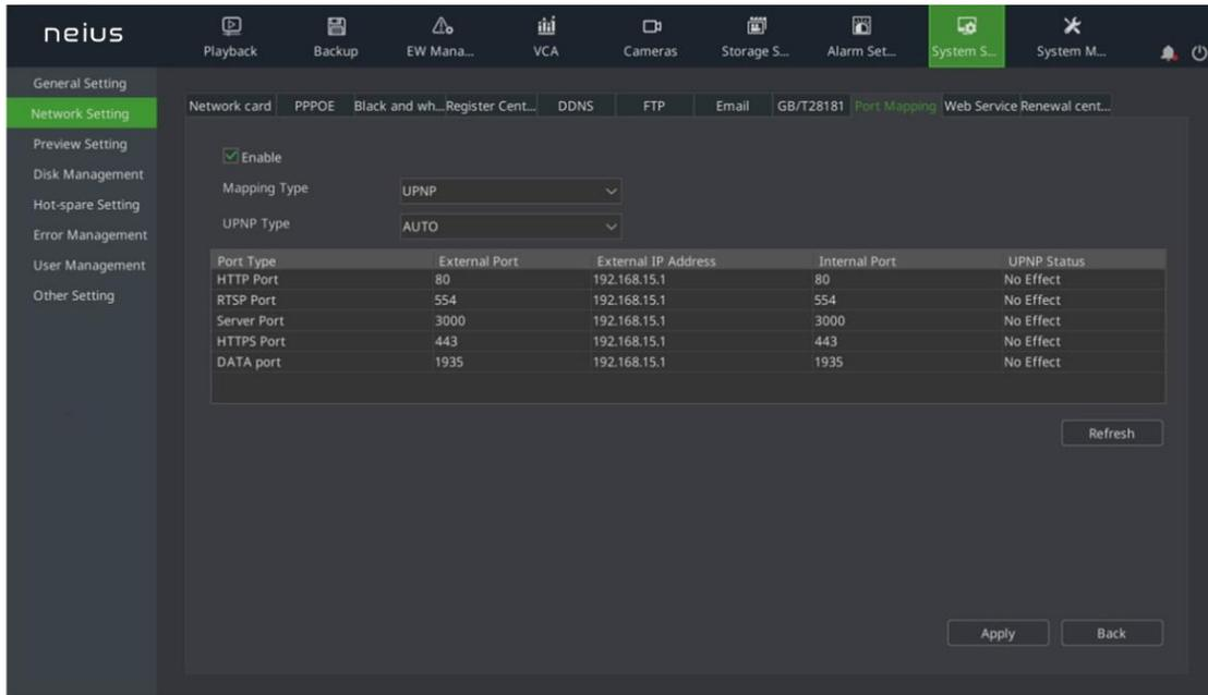
2. Check the “Enable” option to enable “Mapping Type” check box.
