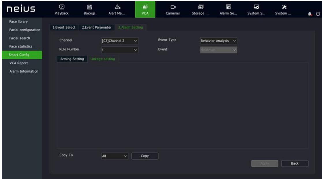
(5) After setting is completed, the parameters of other channels can be copied.
