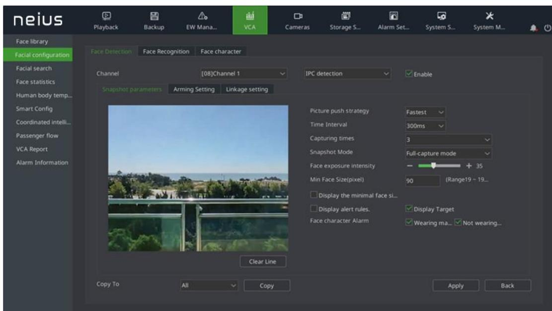
2. Select the algorithm type of face detection, and choose to enable IPC detection /NVR detection.
