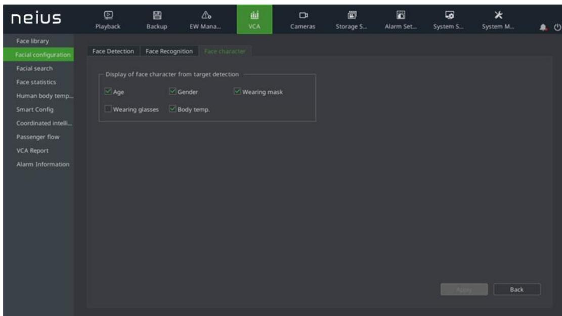
2. Select the face characters in the taskbar of Display of Face Character from Target Detection. At most 4 characters can be selected. View the person identification data in Target Detection.
