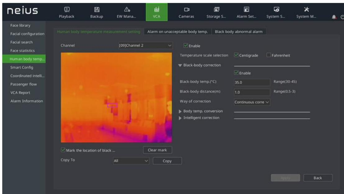
2. The user may set the temperature scale, black body correction, body temp. conversion, etc of the human body measurement according to the needs. The operation procedure is as below:
