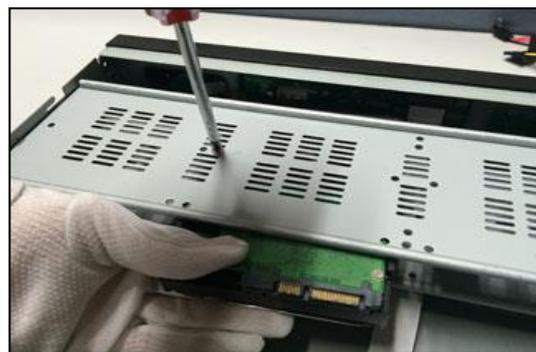
2. Connect one end of the HDD data cable to the SATA interface of the NVR master board, and the other end to the HDD.
