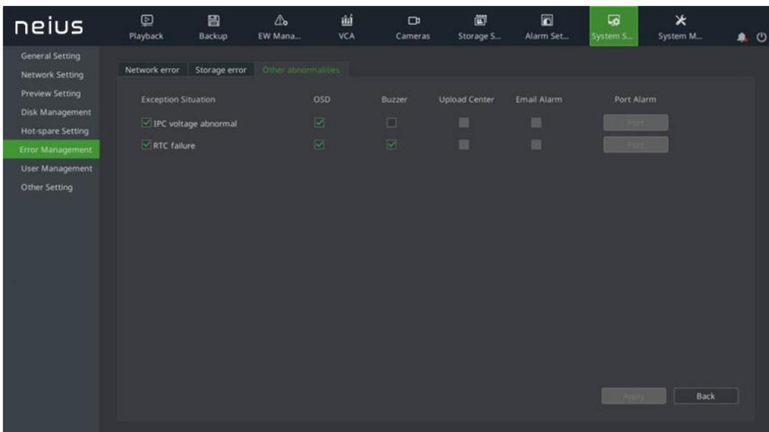
2. After checking the abnormality, the system linkages when the abnormality happens can also be checked, including IPC, abnormal voltage, abnormal RTC, etc.
