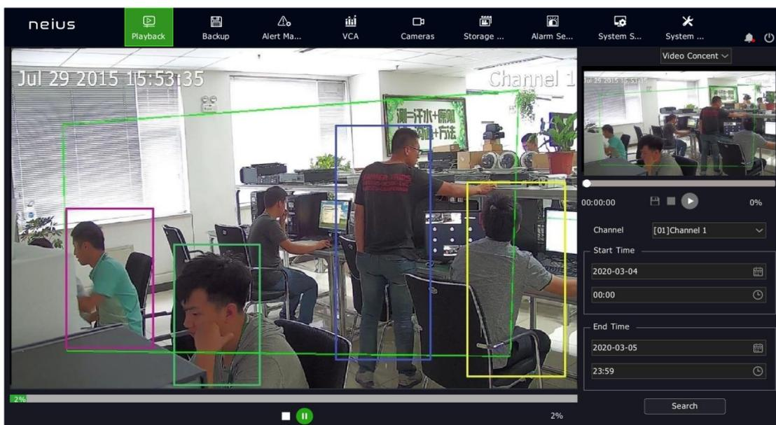
3. Double-click the rectangular box stacked on the left side to locate the time to play in the small window on the right, and then play the video of 30s before and after the time point.
