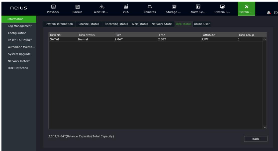
2. HDD number, SMART detection status, size, idle, property, disk pack, total remaining capacity and total capacity of all hard disks can be checked under HDD status.
