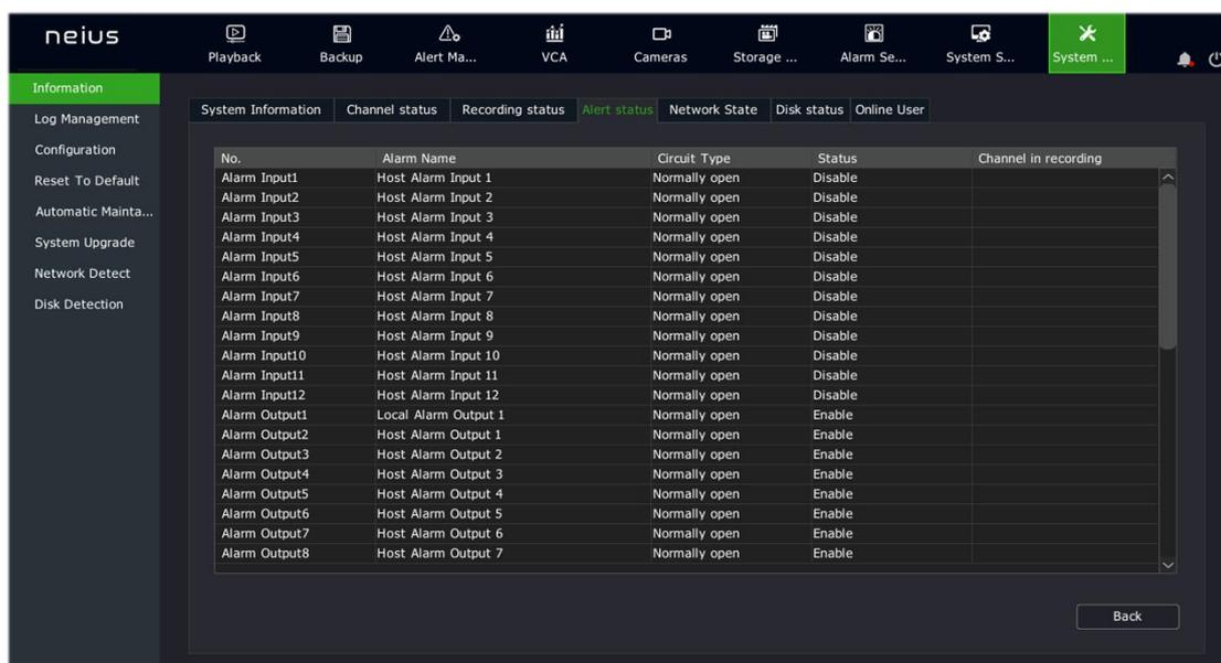
2. Serial number, name, annunciator type, ON/OFF status, channel triggering of the local alarm and alarm host can be checked under Alarm Status.
